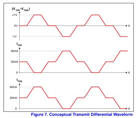
The magnetics module that is external to the 82555 converts  $I_{TDP}$  and  $I_{TDN}$  to 2.0  $V_{pp}$ , as required by the TP-PMD specification. The same magnetics used for 100BASE-TX mode should also work in 10BASE-T mode. The following is a list of current magnetics modules available from several vendors:
